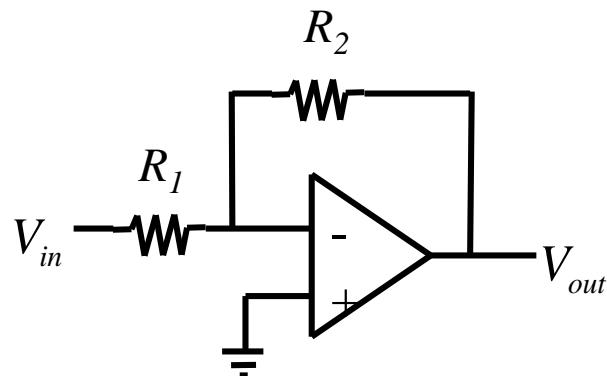
$$K_F = \frac{V_{out}}{V_{in}} = -\frac{R_2}{R_1}$$
