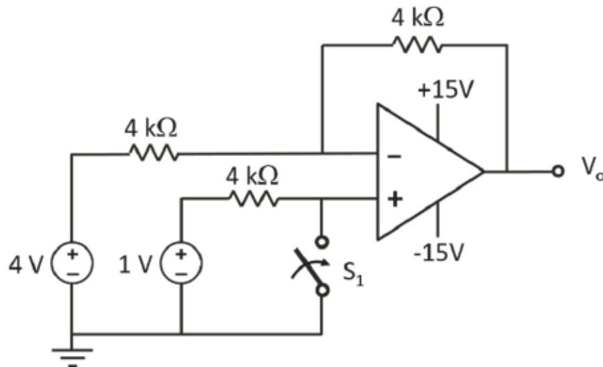
Assuming ideal op amp, determine an expression for the output voltage,  $V_o$ , in terms of the inputs,  $V_1$ , and  $V_2$ .
