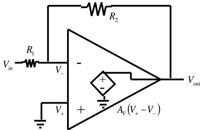
$$K_F = \frac{V_{out}}{V_{in}} = -\frac{1 - \left[ \frac{R_1}{R_1 + R_2} \right]}{\frac{1}{A_V} + \left[ \frac{R_1}{R_1 + R_2} \right]}$$
