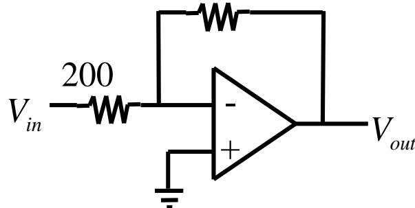
$$\begin{aligned} A_F &= \frac{V_{out}}{V_{in}} \\ &= -\frac{1.245k}{200} \end{aligned}$$
