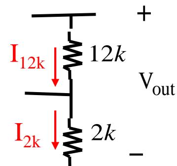
$$\begin{aligned} V_{out} &= (12k + 2k) * 6m \\ &= 84V \end{aligned}$$
